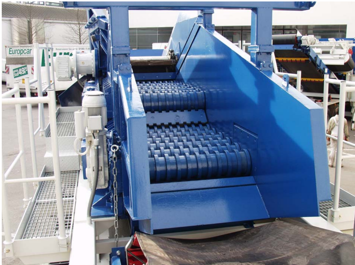
View of the two primary wobbler feeders with step for rearranging the material.
