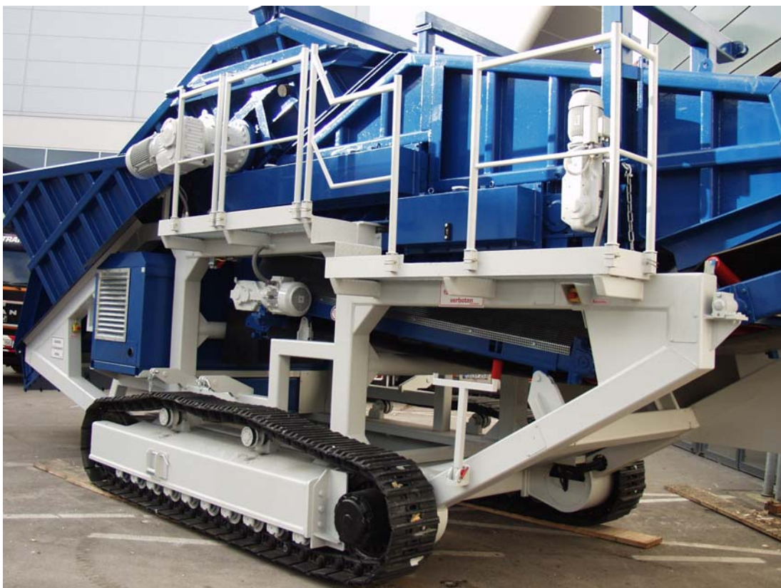
Crawler-mobile Preclassifying Unit Type MOBIDISC MD 10 RR
